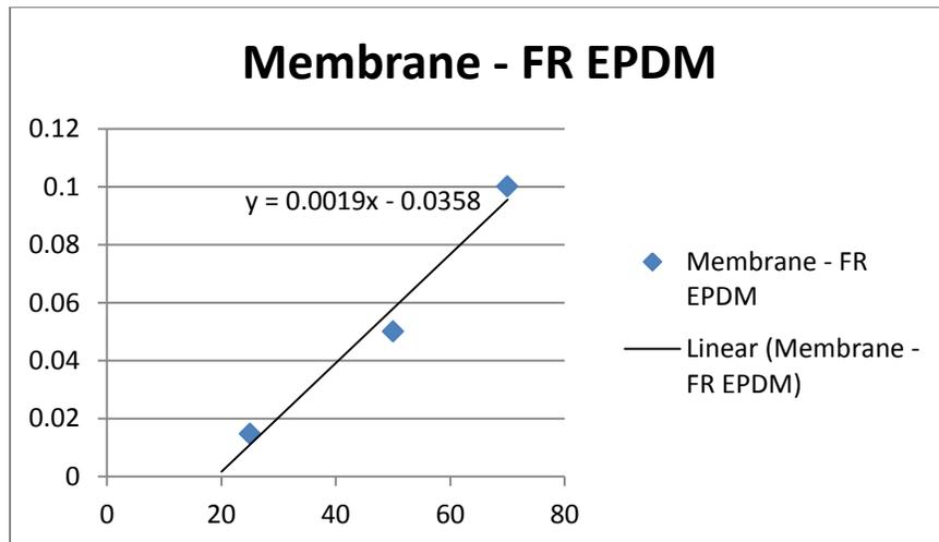
Figure 15 - Graph of 1 / Time to Ignition Vs Heat Flux in kilowatts/m<sup>2</sup>
