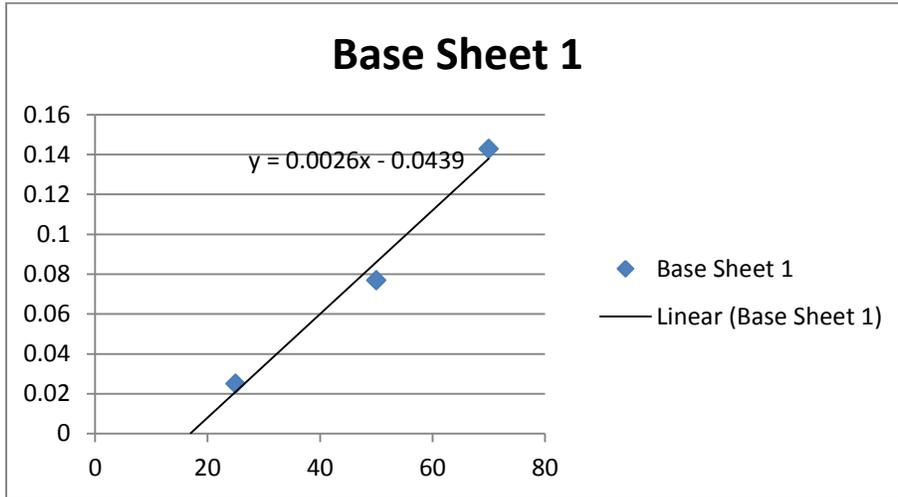
Figure 11 - Graph of 1 / Time to Ignition Vs Heat Flux in kilowatts/m<sup>2</sup>
