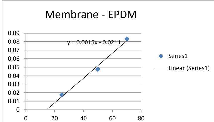
Figure 14 - Graph of 1 / Time to Ignition Vs Heat Flux in kilowatts/m<sup>2</sup>
