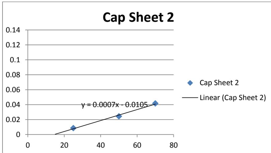
Figure 13 - Graph of 1 / Time to Ignition Vs Heat Flux in kilowatts/m<sup>2</sup>
