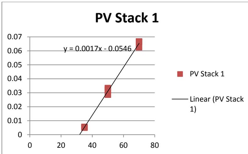
Figure 19 - Graph of  $1 / \text{Time to Ignition}$  Vs Heat Flux in kilowatts/m<sup>2</sup>
