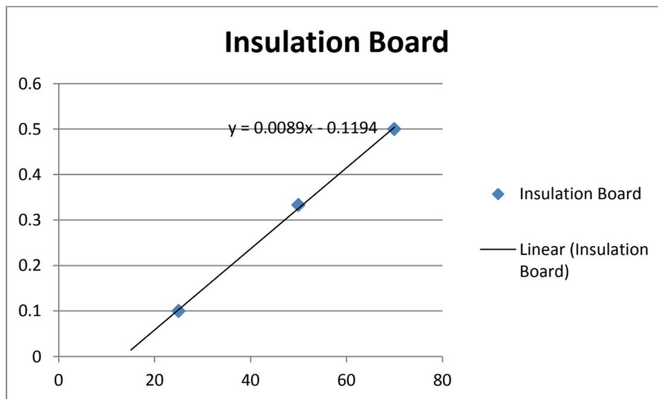
Figure 17 - Graph of 1 / Time to Ignition Vs Heat Flux in kilowatts/m<sup>2</sup>
