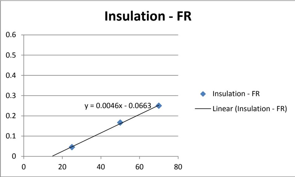
Figure 18 - Graph of 1 / Time to Ignition Vs Heat Flux in kilowatts/m<sup>2</sup>
