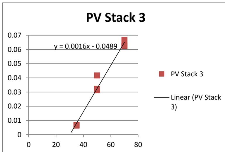
Figure 21 - Graph of  $1 / \text{Time to Ignition}$  Vs Heat Flux in kilowatts/m<sup>2</sup>
