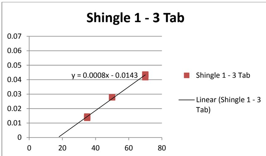
Figure 5 - Graph of  $1 /$  Time to Ignition Vs Heat Flux in kilowatts/m<sup>2</sup>
