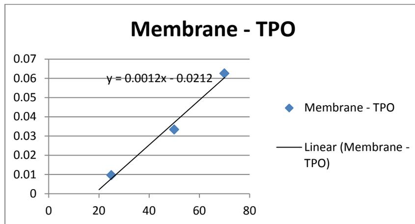
Figure 16 - Graph of 1 / Time to Ignition Vs Heat Flux in kilowatts/m<sup>2</sup>
