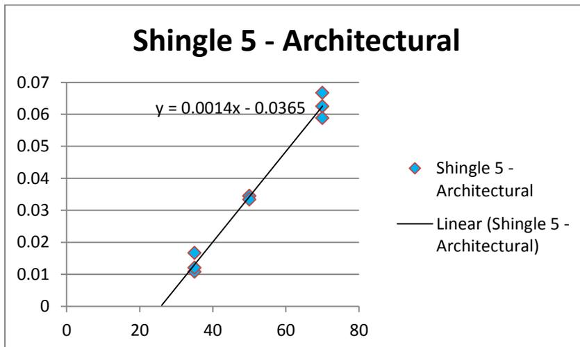
Figure 9 - Graph of  $1 / \text{Time to Ignition}$  Vs Heat Flux in kilowatts/m<sup>2</sup>
