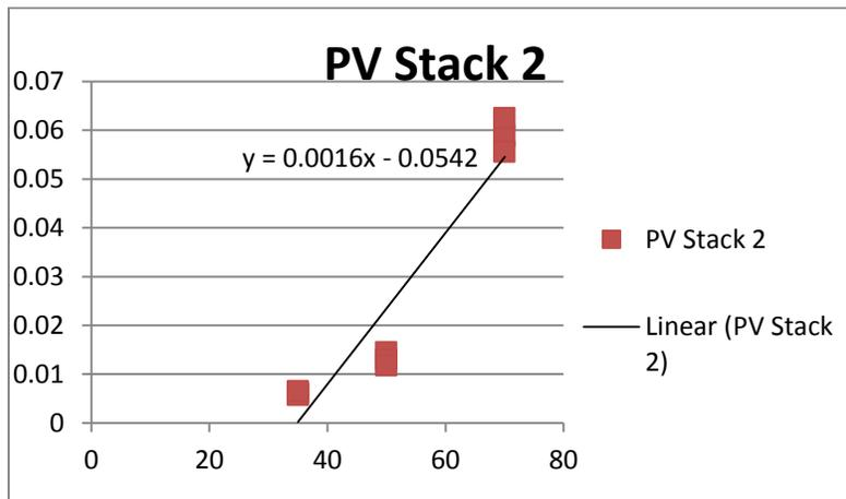
Figure 20 - Graph of  $1 / \text{Time to Ignition}$  Vs Heat Flux in kilowatts/m<sup>2</sup>
