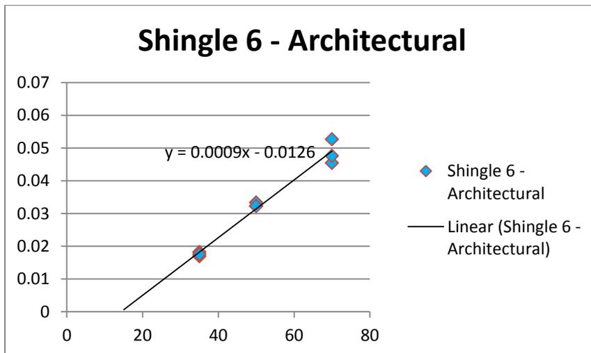
Figure 10 - Graph of  $1 / \text{Time to Ignition}$  Vs Heat Flux in kilowatts/m<sup>2</sup>
