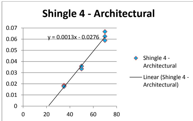
Figure 8 - Graph of  $1 / \text{Time to Ignition}$  Vs Heat Flux in kilowatts/m<sup>2</sup>
