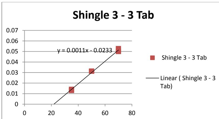
Figure 7 - Graph of  $1 /$  Time to Ignition Vs Heat Flux in kilowatts/m<sup>2</sup>
