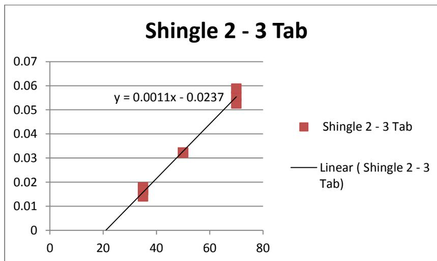
Figure 6 - Graph of  $1 /$  Time to Ignition Vs Heat Flux in kilowatts/m<sup>2</sup>
