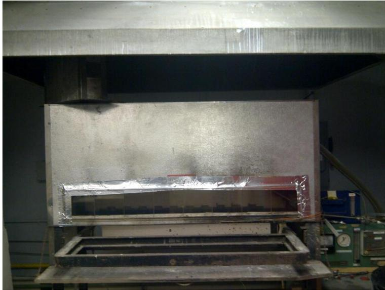
Figure 2 – Figure Illustrates ASTM E1321 LIFT Test Apparatus
