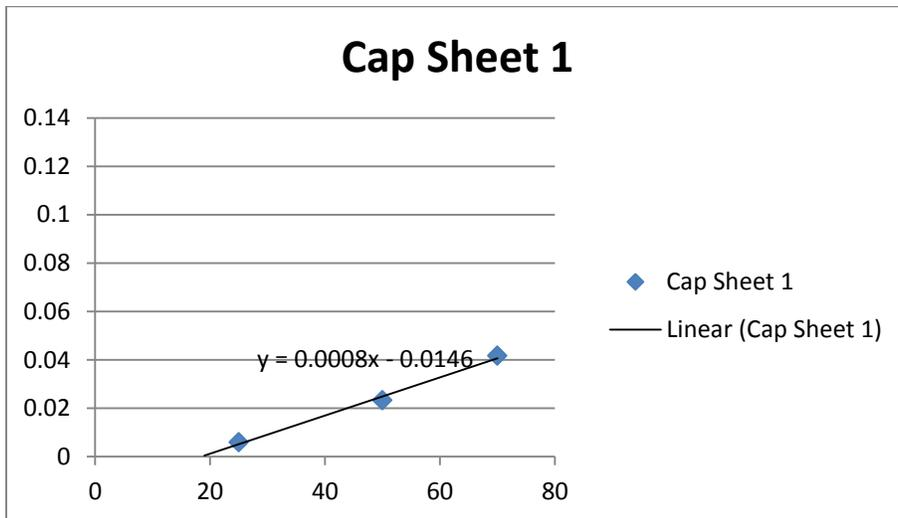
Figure 12 - Graph of 1 / Time to Ignition Vs Heat Flux in kilowatts/m<sup>2</sup>
