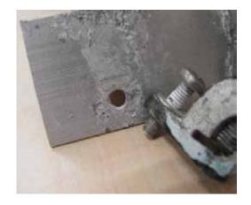
Figure 10 Build-up of white oxidations on the aluminum frame (lug sample)
